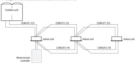
2. Using one wired remote controller to control indoor units connected to different outdoor unit
